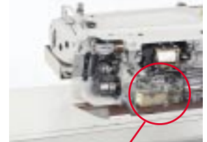
Sealed oil tank
